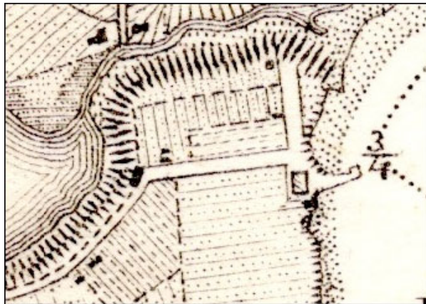
Figure 4: The Anthony-Penfield wharf, as shown on the 1854 Coast Survey map. The number to the right of the wharf indicates that the water depth at the loading dock was 3 to 4 feet.
